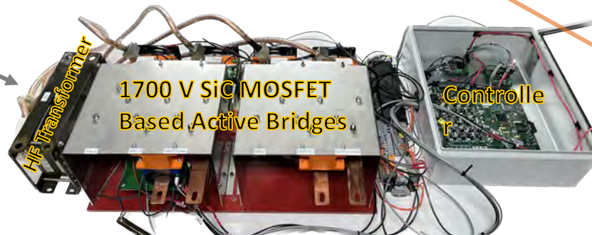
1000 V, 175 kW, 20 kHz DC/DC Charger
