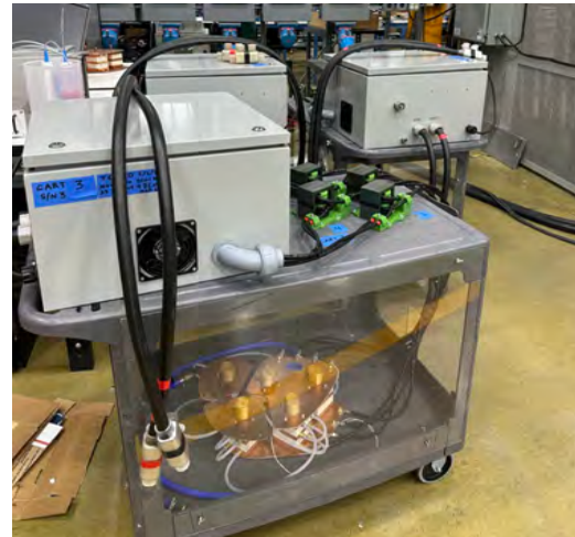
4 primary side HF power electronics units
